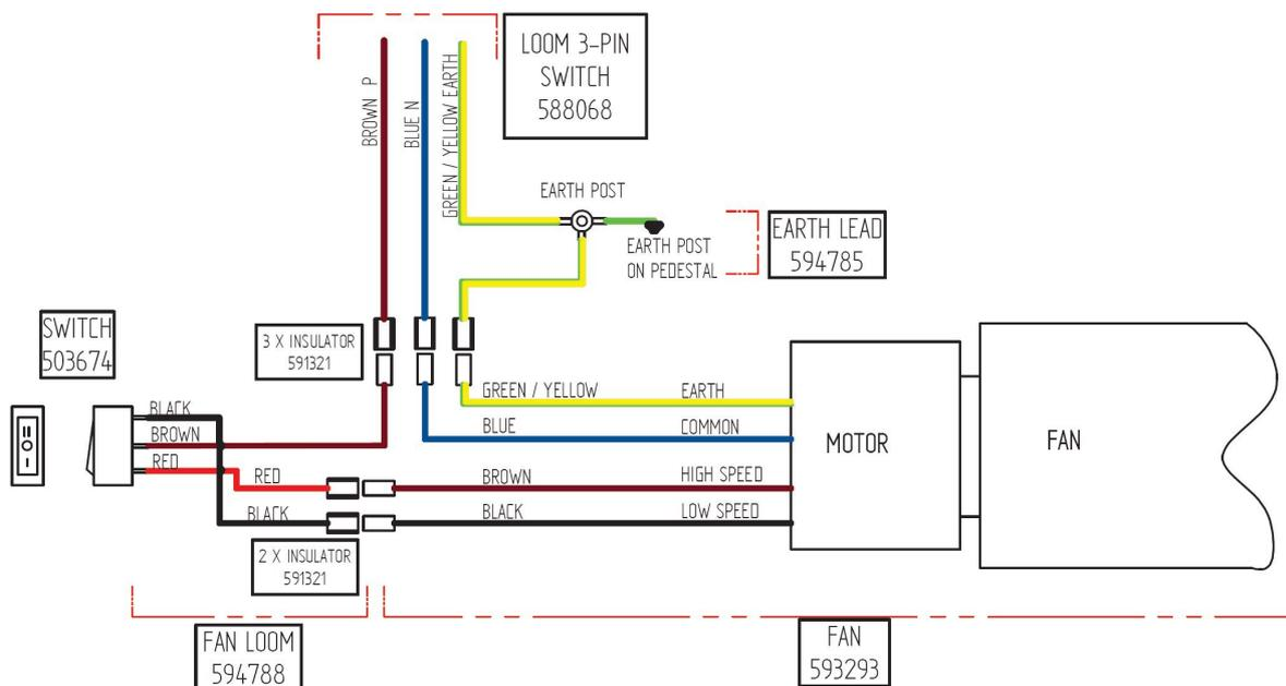
Figure 5. Circuit Diagram—Revision B— 15.11.2013
