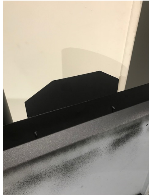
Rear shield plate screwed to rear panel (Screw ends will not be visible when fitted on fire)
