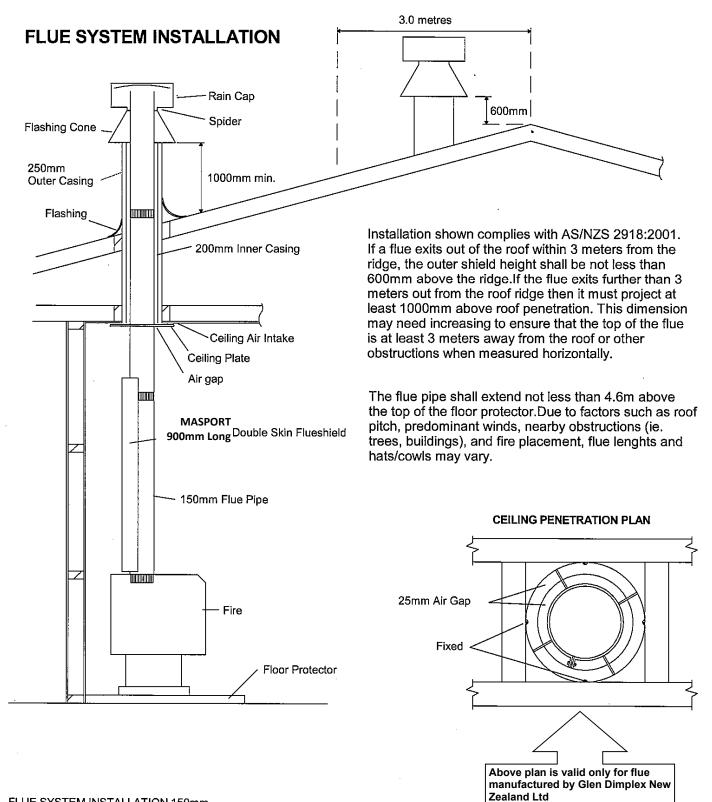
FLUE SYSTEM INSTALLATION 150mm
